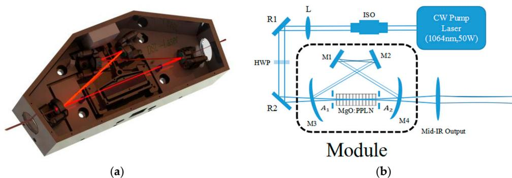
**Figure 1.** The configuration of the module (a) and the optical schematic of the experiment (b). HWP: half wavelength plate; ISO: isolator; MgO:PPLN: MgO-doped periodically poled lithium niobate crystal; CW: continuous-wave.
