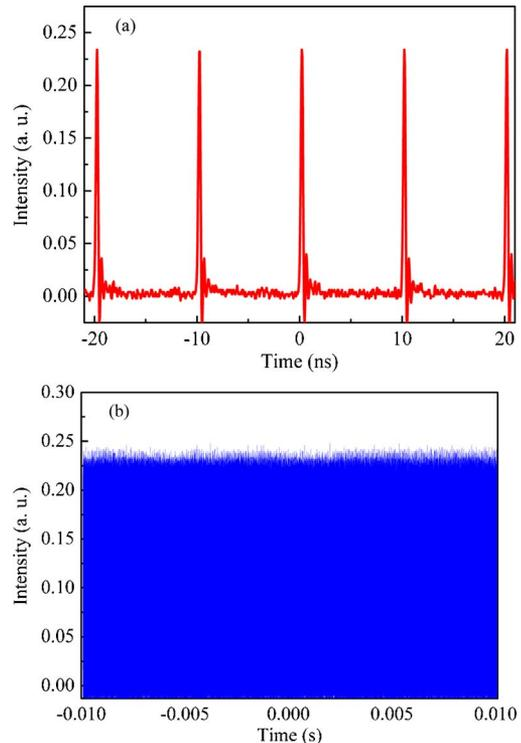
Fig. 3. (Color online) Captured waveform of the pulse train: (a) in nanosecond scale and (b) long-term recording of a cw mode-locked pulse train in millisecond scale.
