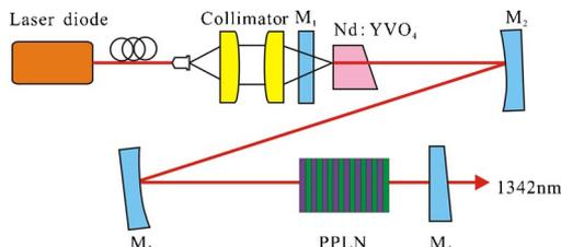
Fig. 1. (Color online) Schematic of NLM mode-locked 1342 nm laser.
