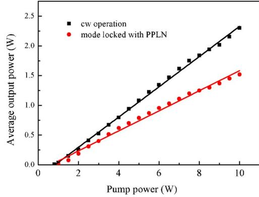
Fig. 2. (Color online) Measured average output power as a function of the incident pumping power in the cw and mode-locked regime.
