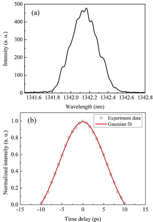
Fig. 4. (Color online) (a) Spectrum of cw mode-locked output and (b) autocorrelation trace of Nd:YVO<sub>4</sub> laser.
