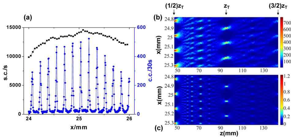
FIG. 2. (a) Measured single counts (black squares) and coincidence counts (blue dots) versus the transverse position of the slit at the first Talbot length  $z_T = 96.2$  mm. (b) Experimental and (c) theoretical two-photon Talbot carpet from  $(1/2)z_T$  (48.1 mm) to  $(3/2)z_T$  (144.3 mm).
