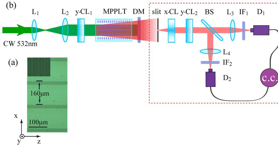
FIG. 1. (a) Micrograph of the etched MPPLT. (b) Experimental setup.  $L_1$ - $L_4$  are convex lenses,  $y$ -CL $_1$  and  $y$ -CL $_2$  are cylindrical lenses focusing along the  $y$ -axis, and  $x$ -CL is a cylindrical lens focusing along the  $x$ -axis.
