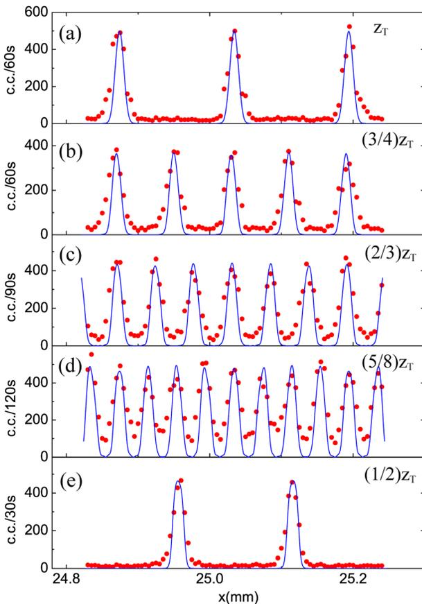
FIG. 3. The red dots are the measured integer two-photon Talbot images detected at distances of (a)  $z_T$ , (e)  $(1/2)z_T$  and fractional images at distances of (b)  $(3/4)z_T$ , (c)  $(2/3)z_T$ , and (d)  $(5/8)z_T$ . The blue lines are theoretical curves.
